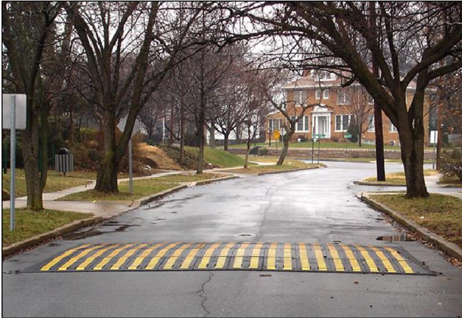
Figure 6 – Temporary Speed Hump
